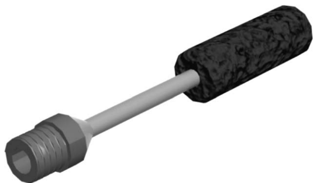
Fig. 1. 60 ppi RVC rotating cylinder cathode.
